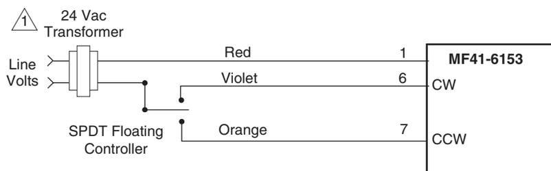
Figure 1 Typical Wiring Diagram for MF41-6153 Floating Actuators.
