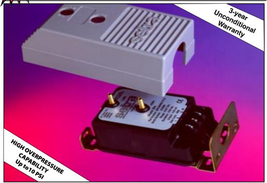
etra Systems 264 pressure transducers sense differential or gauge (static) pressure and convert this pressure difference to a proportional electrical output for either unidirectional or bidirectional pressure ranges. The 264 Series is offered with a high level analog 0 to 5 VDC or 4 to 20 mA output.
