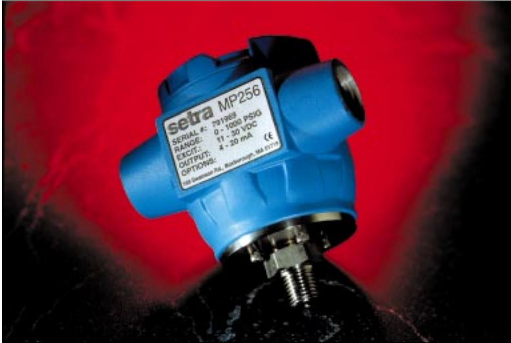
Setra's Model 256 industrial pressure transducer is one of the most rugged and reliable sensors available. The Model 256 is packaged in a die-cast aluminum enclosure that is specifically designed for NEMA4/IP65 service. Setra's robust capacitive design is resistant to environmental effects, such as shock, vibration, temperature and EMI/RFI. Setra's all stainless steel sensing element does not require isolation from corrosive media.
